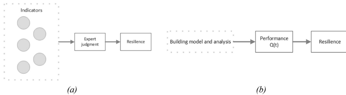
Fig. 8. Schematic of the methodology comparison between the expert-based indirect approach (a) and the direct engineering-based approach (b). [source: authors]
