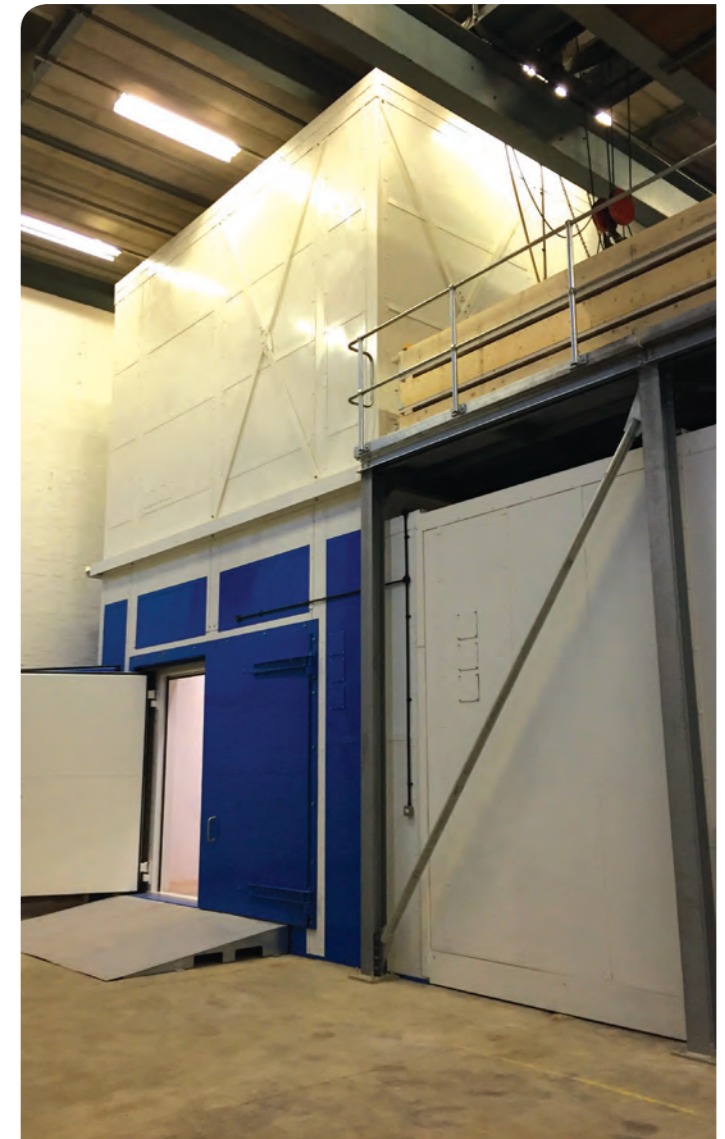
The BRE sound transmission testing suite
