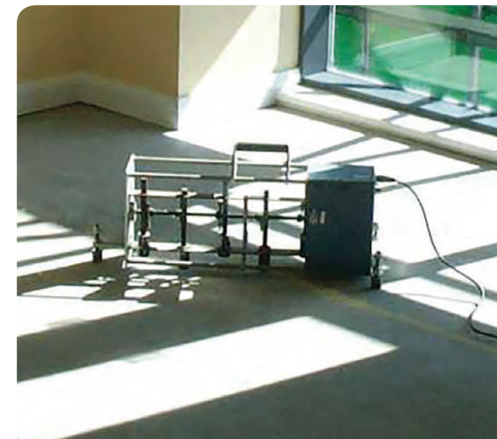
Tapping machine used in sound insulation tests
