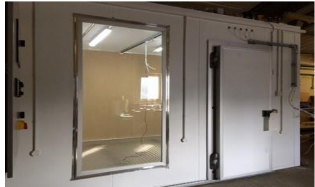
BRE's 30 m 3 'ECO-SEE' environmental chamber (conforms to CEN 16516).
