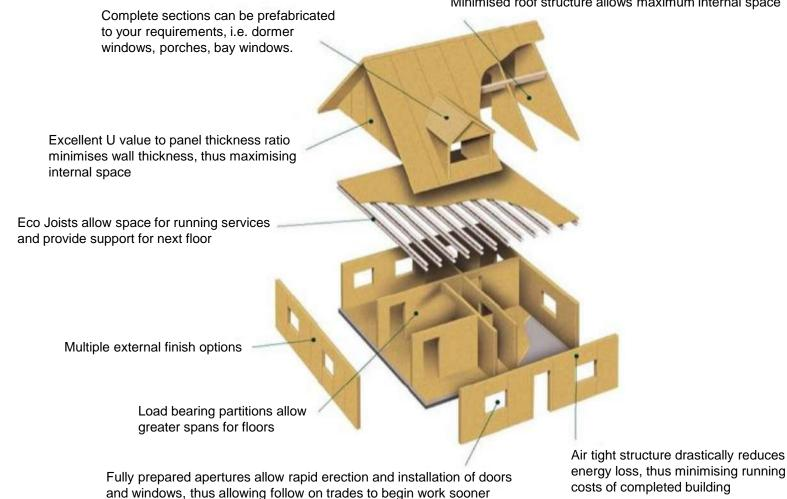
Minimised roof structure allows maximum internal space
