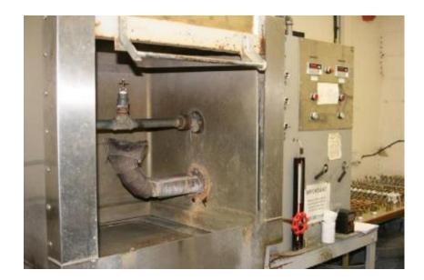
Watermist nozzle test based on sprinkler component tests from EN 12259-1
